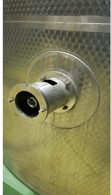
Chemical tank mixer with special hard faced mechanical seal & water flush
