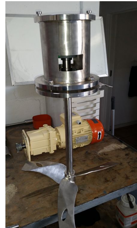
Side-entry mixer on a 50 000L horizontal cold-stabilisation tank, running at - 4C
