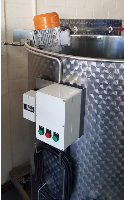
High-speed balie mixer for bentonite slurry make-up
