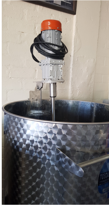
Low-speed balie mixer for yeast slurry make-up.
