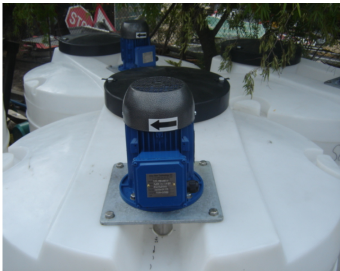
Frame & stand with top-entry mixer for chemical applications.
