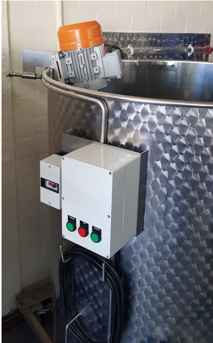
High-speed balie mixer for bentonite slurry make-up
