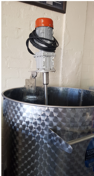
Low-speed balie mixer for yeast slurry make-up.
