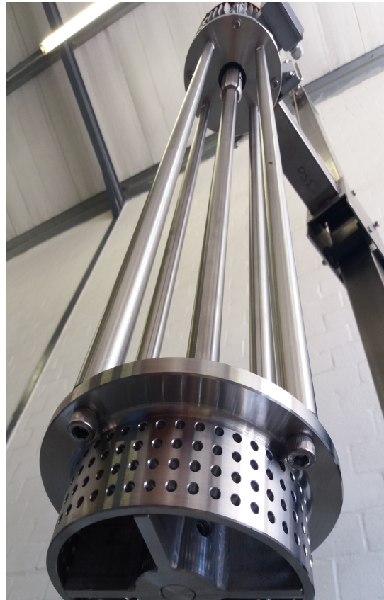
Top and bottom: heavy-duty, top-entry ink milling homogeniser.
