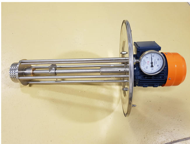
Above: batch processing homogeniser for nut milk make-up complete with analogue-type temperature gauge
