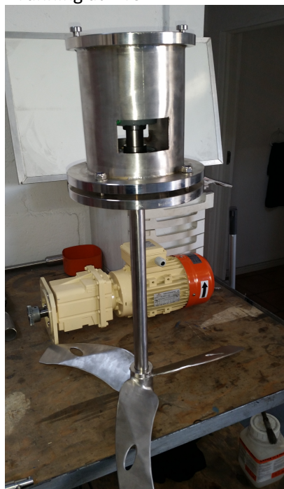
Above: Bayonet-type, portable drive mixer complete, tank bedestal assembly and bayonet coupler
