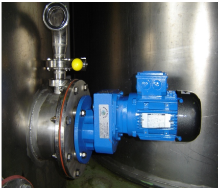
High-efficiency side-entry mixer on a syrup blending application
