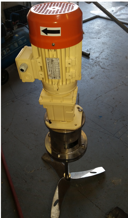
Above: Bayonet-type, portable drive mixer complete, tank bedestal assembly and bayonet coupler
